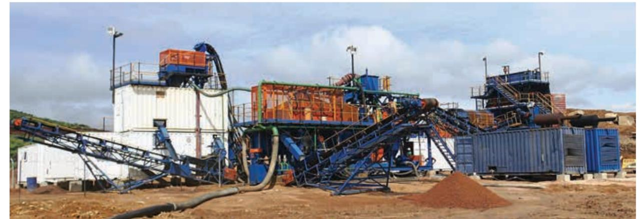
The Baoulé 100 t/h DMS plant is able to treat both fresh and weathered kimberlite ore.
